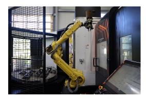
(Halter\_CNC\_Automation\_02 METAV Automation an WZM.jpg) One of the three loading robots at Heinz Knöpfle GmbH coupled to a CNC turning/milling center. Photo: Richard Pergler
