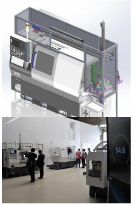
(Citizen\_Machinery\_Europe\_01 METAV Automation an WZM Gantry Loader.jpg) High-precision lathe with gantry loader. Customers can use position tables to carry out free horizontal and vertical programming of the gantry axes. This facilitates the use of a highly flexible range of workpieces and allows fast changeovers. Accuracies of ±0.02 mm can be achieved when positioning the workpieces. Photo: Citizen Machinery Europe GmbH
