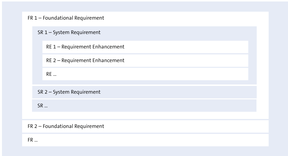
Fig. 19: Hierarchy of requirements in IEC 62443-3-3
