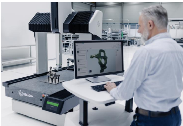
The latest coordinate measuring machine from Hexagon works with the I++ DME standard. (Foto: Hexagon)
